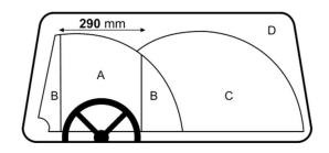
The following size of windscreen chip damage can be repaired in accordance with the British Standard Code of Practice BS AU 242a:1998
